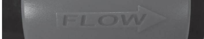
2. Determine the ideal mounting location for the fuel pump, a secure location like the frame is ideal. The fuel pump must be mounted at or below the lowest point of the fuel tank. The pump must also be within one foot of the fuel tank as it's designed to push fuel from the tank towards the engine. **WARNING: Fuel pump failure will occur if not mounted within the required specification.**
