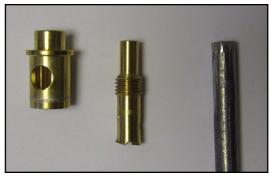
Modify a atomiser by removing the head with the screw driver slot, using a hack saw cut a slot across the new end suitable for a screwdriver.
