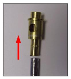
Wind the modified atomiser into the bush from the float bowl side until all the threads are engaged, normally about 5 turns.
