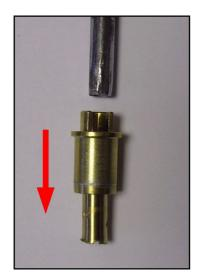
Wind the modified atomiser into the new bush as before, working from the top of the carburettor. Align the bush with hole in the carburettor body, ensuring the hole in the side of the bush is aligned with the corresponding hole in the body, bushes that have a raised shroud should also have the lowest edge, or the cut-out squarely aligned with the engine end of the carburettor.
