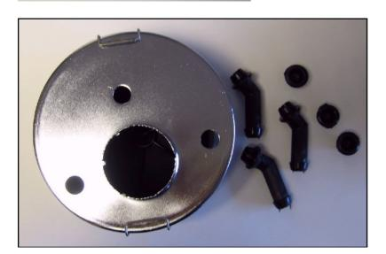
Fitting to Dellorto carburettors with a pump diaphragm.
