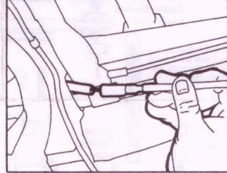
Slide the steel cable end firmly over the stock throttle cable tube that runs through the car.
