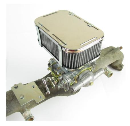
Re-fit the locking washer and nut. Tighten the nut by hand and then 1 additional flat with a spanner, bend locking washer tab to lock nut in place.
