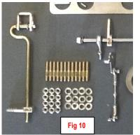
With the aluminium clamp lever loose on the shaft, push the bar into the bulkhead support bush. Push U shaped coupling (Fig 10) over the 2 flats on the threaded end of the cross shaft. Fit washer. Tighten Staytite nut.
